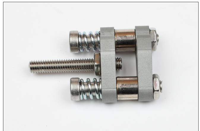
Figure 27: The screws are loosened with 3 turns (M6 has a lead of 1 mm/turn), and then locked in this position with the lock nut.
