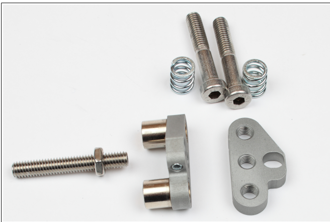
Figure 23: The headless hexagonal socket screw M6x40 is removed.
