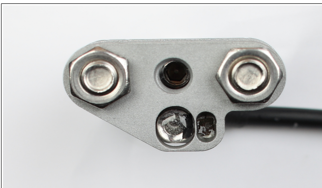
Figure 30: Note that the black Hall effect sensor element faces the magnet. The Hall effect sensor element is the black part inside the nickel-plated sensor bushing. The magnet is glued in the the magnet plate.
