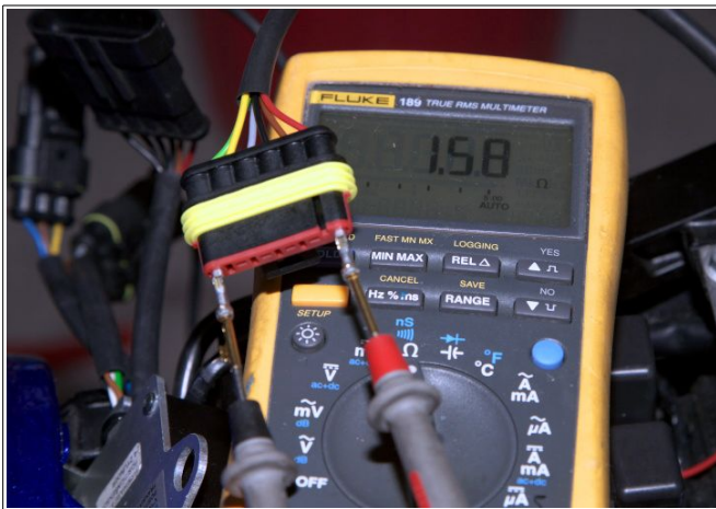
Figure 10: Measurement of the ignition coil resistance.
