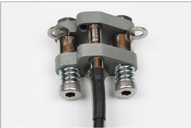
Figure 29: The Hall effect sensor is adjusted (in regard of the minimal triggering force), at which the sensor should be pre-loaded with about 1 mm. With reaching the minimal triggering force, the “force” (or “start”) LED lights up.
