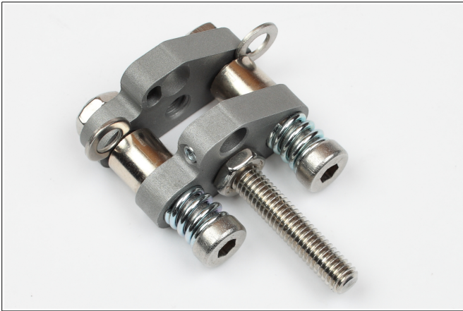
Figure 28: The sensor is pre-loaded with 1 mm. For this purpose, M5 washers, which have a thickness of 1 mm, are suited.
