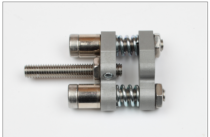
Figure 20: The Hall effect sensor is removed (with hexagonal socket wrench of wrench size 2).
