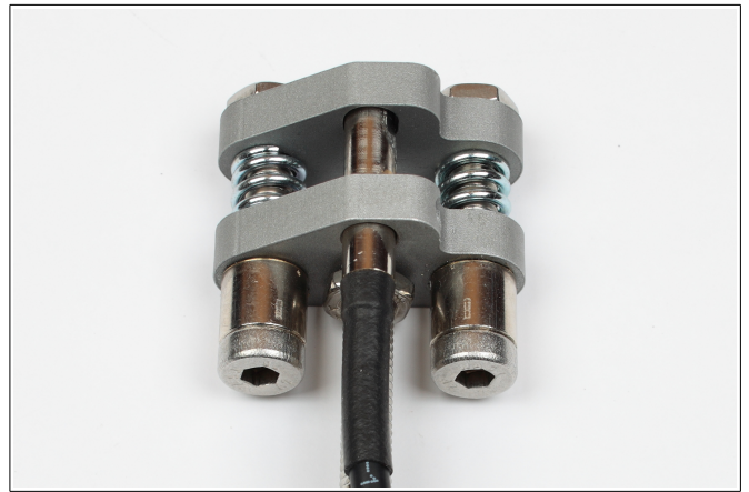
Figure 19: The force sensor is put together as pressure sensor. The springs are within the plates.
