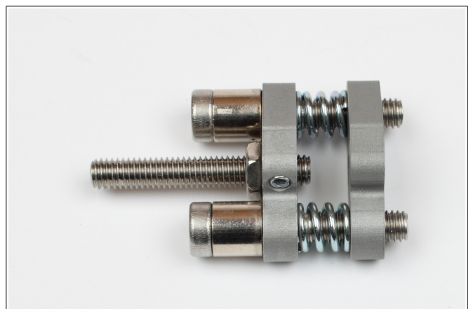
Figure 21: The lock nuts are loosened and removed (wrench size 10).
