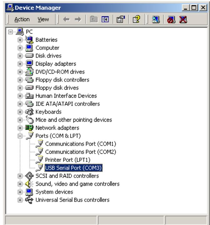
Figure 1: USB SER port in the Windows Device Manager.
