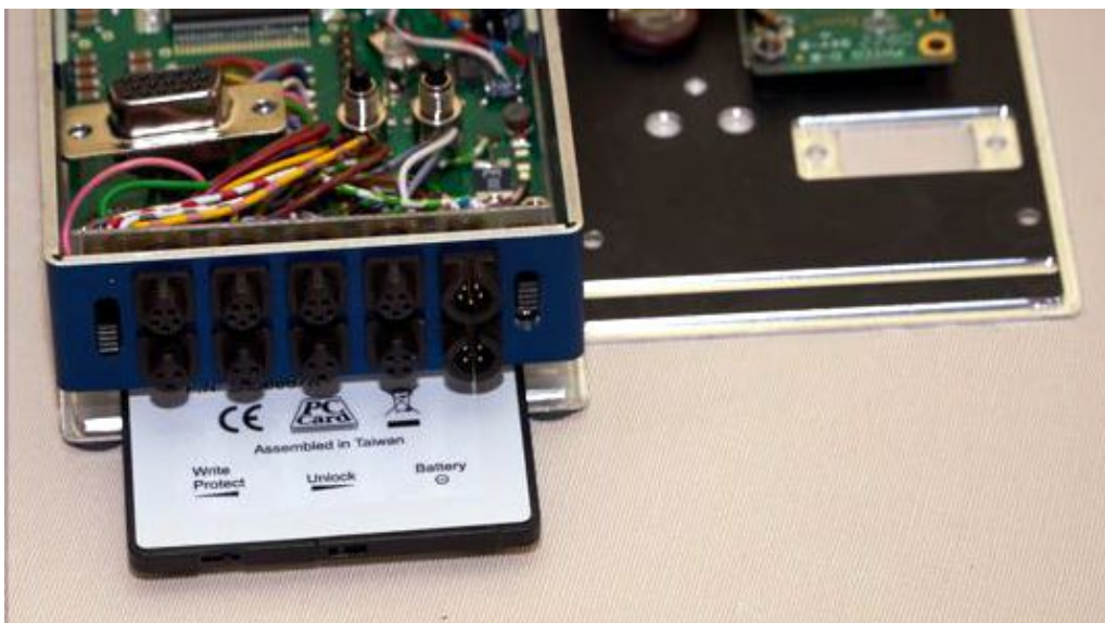
Figure 5-4: Remove the card. The card can be levered with a screwdriver (by using the notches).
