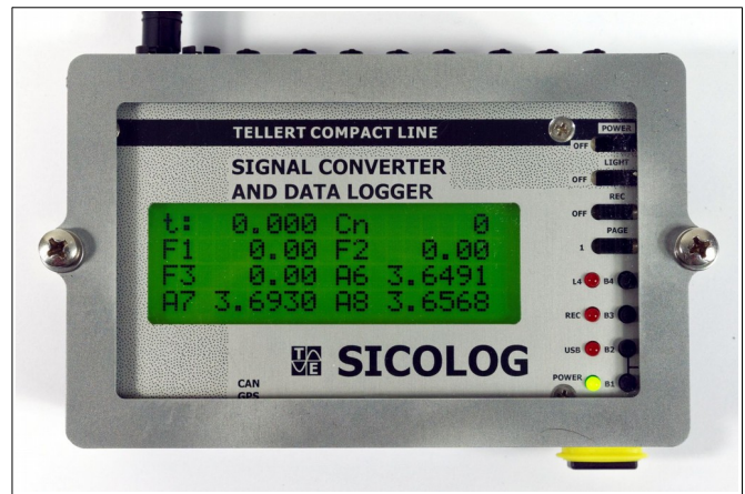
Figure 2: SICOLOG with splash water protection.
