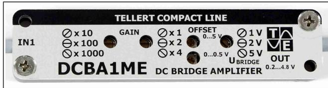
Figure 1: DC Bridge Amplifier DCBA1ME.
