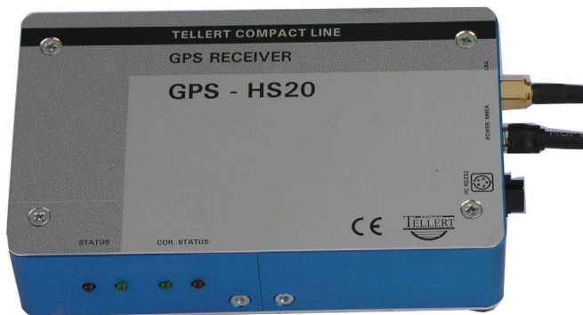
Figure 1: GPS receiver GPS-HS20.
