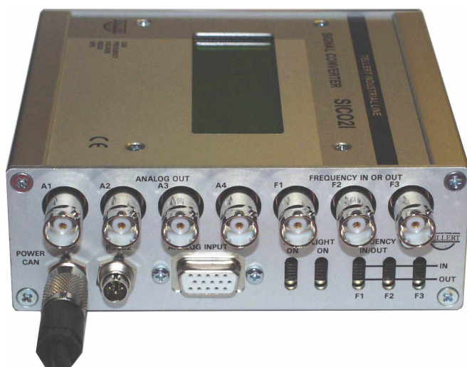
Figure 3: Signal converter SICO2I (Connectors).
