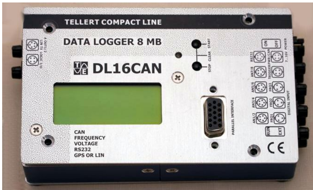
Figure 5-1: Unscrew the four M2.5 screws from the lid and the two M2.5 screws from the parallel interface.
