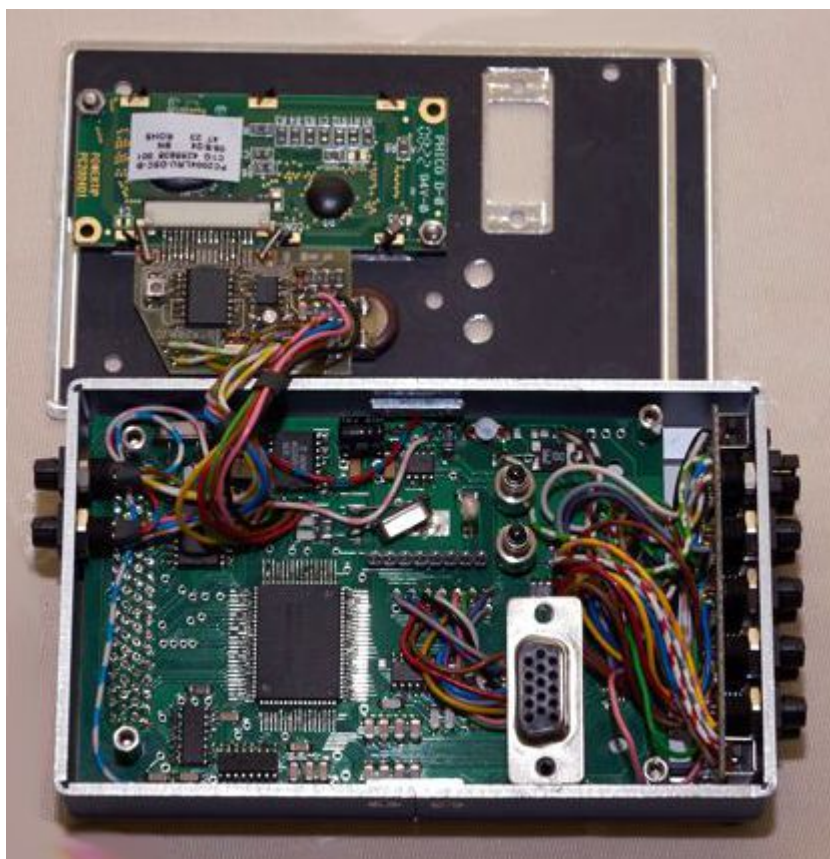
Figure 5-2: Turn the lid to the top. (Pay attention that the LED is adjusted correctly, and that the wires don't occupy the space for the MCU when closing the lid).
