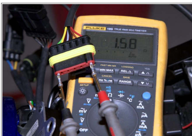
Figure 10: Measurement of the ignition coil resistance.
