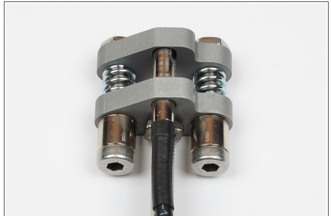
Figure 18: The force sensor is put together as pressure sensor. The springs are within the plates.
