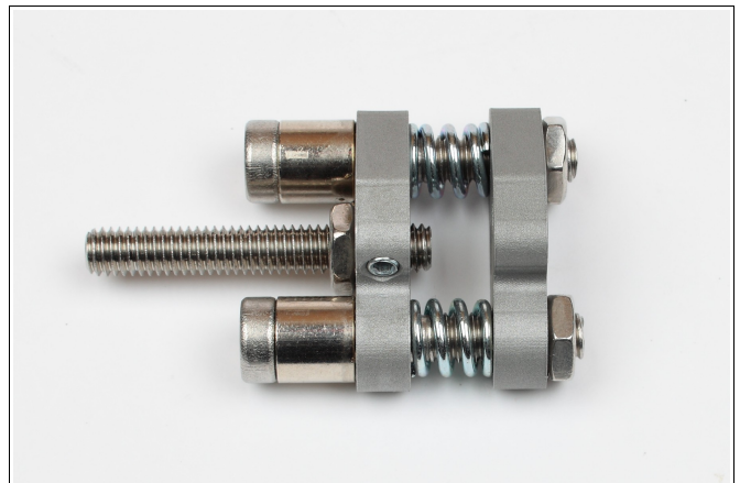
Figure 19: The Hall effect sensor is removed (with hexagonal socket wrench of wrench size 2).
