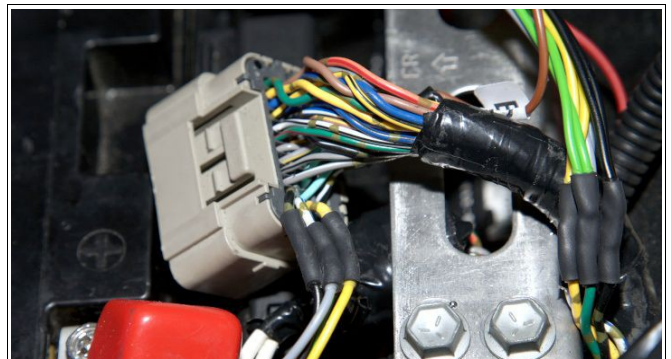
Figure 7: CTS connection with the ECU connector 1/3.
