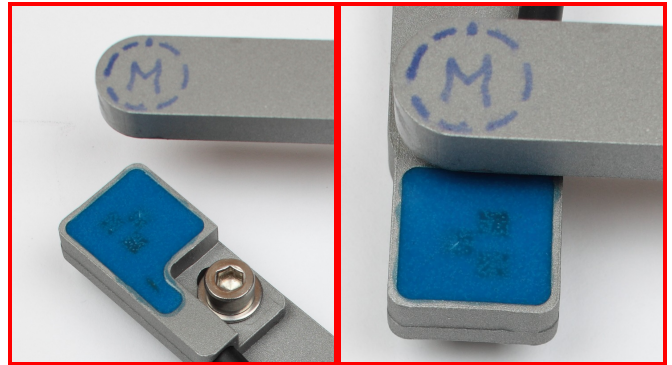
Figure 41: Wrong arrangements – the sensor element paws are partially in contact signals first (left); the sensor element end stop signals first (right);
