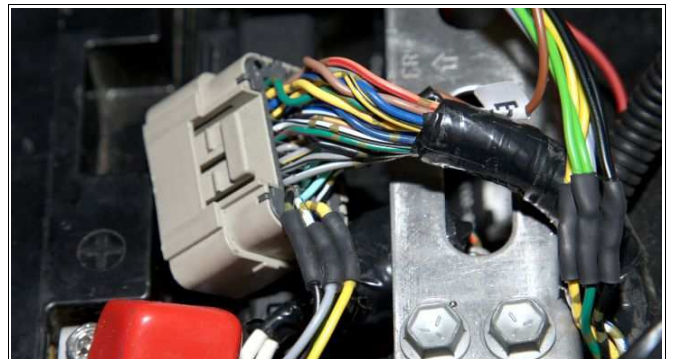
Figure 7: CTS connection with the ECU connector 1/3.
