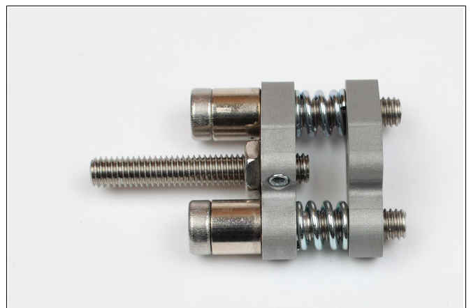
Figure 20: The lock nuts are loosened and removed (wrench size 10).
