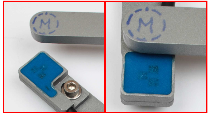
Figure 38: Wrong arrangements – the sensor element paws are partially in contact signals first (left); the sensor element end stop signals first (right);
