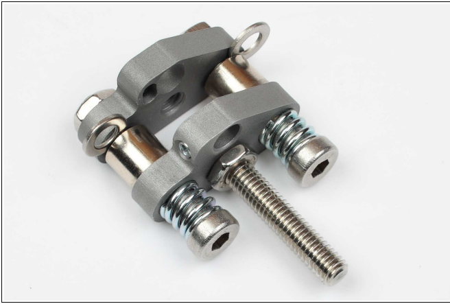
Figure 27: The sensor is pre-loaded with 1 mm. For this purpose, M5 washers, which have a thickness of 1 mm, are suited.
