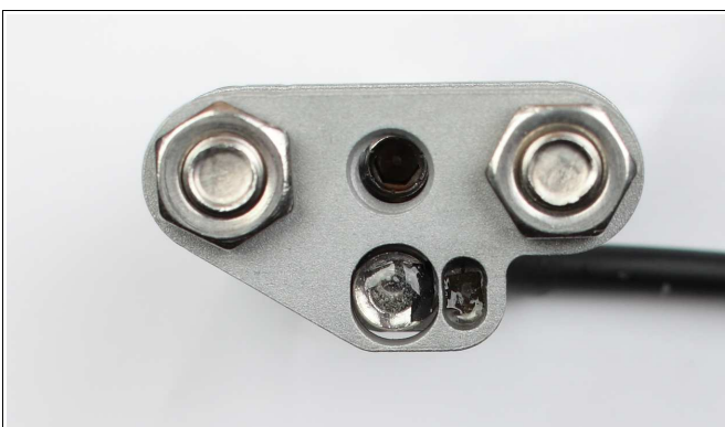
Figure 29: Note that the black Hall effect sensor element faces the magnet. The Hall effect sensor element is the black part inside the nickel-plated sensor bushing. The magnet is glued in the magnet plate.
