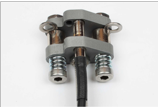
Figure 28: The Hall effect sensor is adjusted (in regard of the minimal triggering force), at which the sensor should be pre-loaded with about 1 mm. With reaching the minimal triggering force, the “force” (or “start”) LED lights up.
