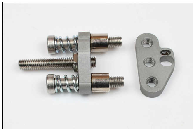
Figure 24: The springs are put on the screws.
