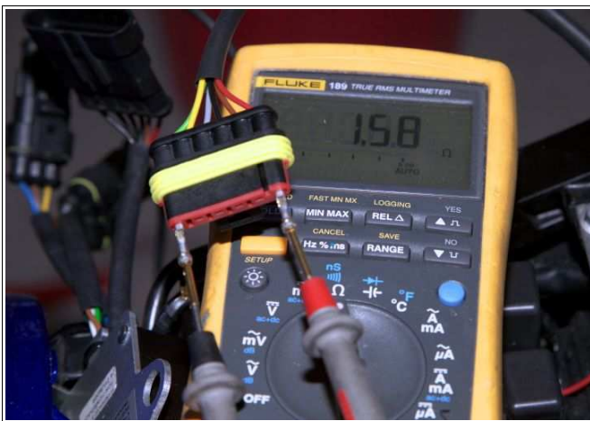
Figure 10: Measurement of the ignition coil resistance.
