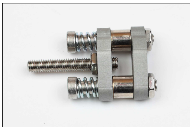
Figure 26: The screws are loosened with 3 turns (M6 has a lead of 1 mm/turn), and then locked in this position with the lock nut.
